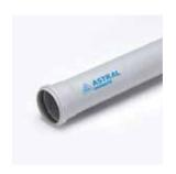
**SELFIT** PIPES: (Type A & Type B): Selfit pipes are socketed on automatic socketing machine with self socket length (without groove). Such pipes are to be joined with solvent cement. One end of the pipe is plain and the other is self socketed on sophisticated automatic machines for high degree of accurate diameters. The pipes when joined using solvent cement, form a permanent water tight joint.
