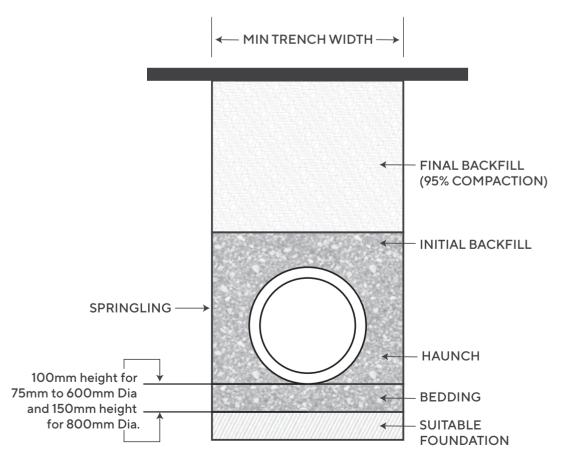
Figure 7: Cross Section of a Typical Trench
